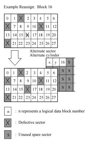
Figure 3.8 Alternate block allocation by REASSIGN BLOCKS command
